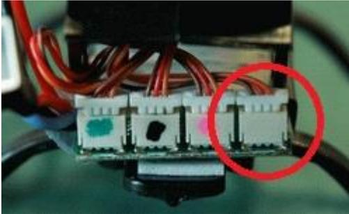
**Step 2** - Thread the servo lead from your new Lynx DS-883 servo into the 130X frame and connect to the 3-in-1 control board. As the servo leads pass through the forward section of the frame, thread the servo leads out and back into the frame, where they pass under the battery and around the motor (as illustrated below). This will keep your servo wires back away from the motor and avoid both rubbing and damage from heat.
