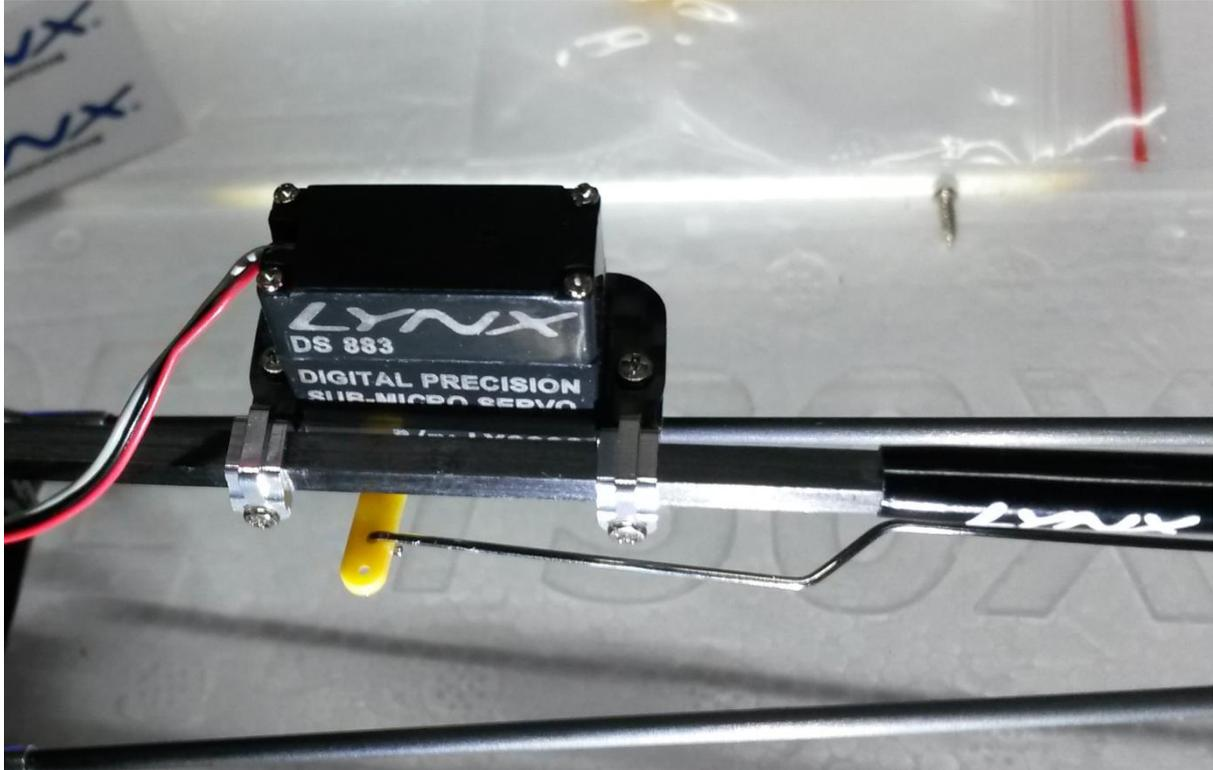
**Step 4** - Connect your 130X tail pushrod to your new Lynx DS-883 servo. Give the pushrod a quarter turn in the ball-link to line up with the servo arm, and hook it onto the servo arm, as shown below. You need to select a servo horn and hole position that will position the pushrod approximately 5.5mm out from the centre.
