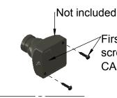
First removed the 2 STD screws and leave the CAM plate in place
