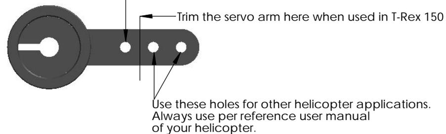
NOTE: During assembly this screw must lock loose, otherwise the servo arm cannot rotate in case of crash. We suggest locking the screw completely, and then open half of turn. This operation is mandatory for the perfect function of the system.
