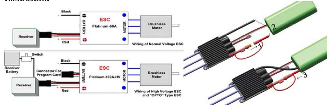
The Platinum-150A-OPTO, Platinum-70A-HV, Platinum-120A-HV, Platinum-80A-HV and Platinum-100A-HV ESC use the new anti-spark structure.
