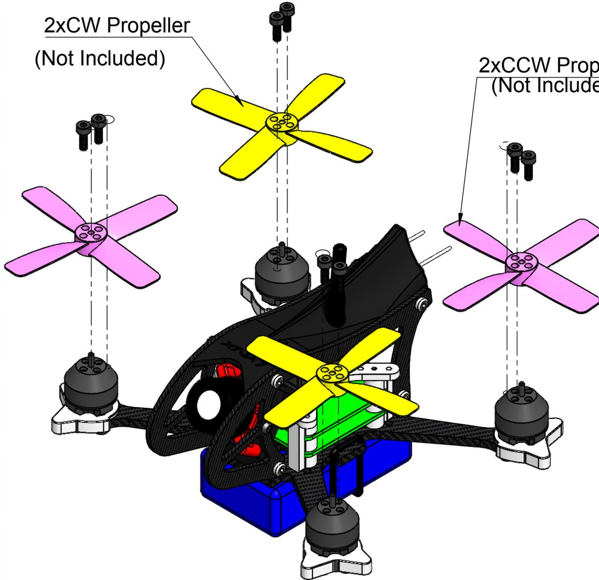
Note rotation direction of the Propeller
